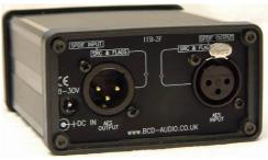
If the SRC is selected, the S/PDIF output is clocked from the S/PDIF input, completely isolating the Consumer side from the Professional side.
